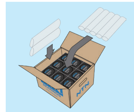
Fig. 6.38 Transportation and storage by shipping box
