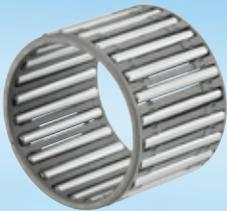
A needle cage comprises an inseparable cage and needles and can be used to design very compact, light, constructions with maximum capacity. The shaft and housing act as a raceway and must be machined in compliance with hardness, geometry and roughness characteristics. The needles are guided precisely, therefore the needle cage can absorb much higher speeds of rotation than contact needles.
