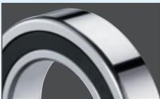
Nitrile seals fixed on the outer ring, with no contact with the inner ring, can be used to maintain the same maximum speed as with an open bearing, lubricated with grease.
