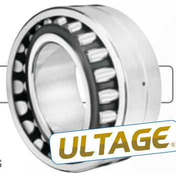
This unit compensates for shaft bending and absorbs misalignment defects. These accept high radial loads and axial loads in both directions. Available with tapered or cylindrical bores. Tapered bores are delivered with adapter or withdrawal sleeves.
