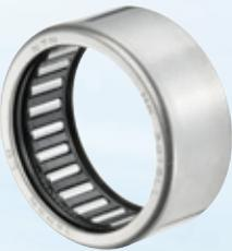
Compact and light, mainly used in applications with low loads, needle sockets represent a low-cost bearing solution; the outer ring is not machined, but is obtained using precision pressing processes. It must be noted that the geometry of the raceway depends on the geometry of the housing (the low thickness of the outer ring only provides the hardness and roughness necessary for the raceway).
