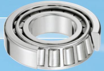
These accept high radial loads and axial loads in one direction. They are generally fitted opposite a bearing of the same type. Load capacity depends on contact angle.
