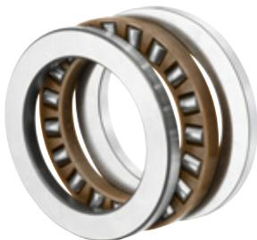
**Needle or roller thrust bearings are designed to absorb axial forces in one direction only. Support surfaces used as raceways must be ground and hardened.**
