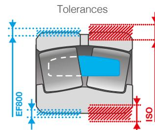
Reduced bore tolerances for cylindrical, tapered and for the outer diameters compared with tolerance ranges of standard series, guaranteeing perfect ring adjustment.
