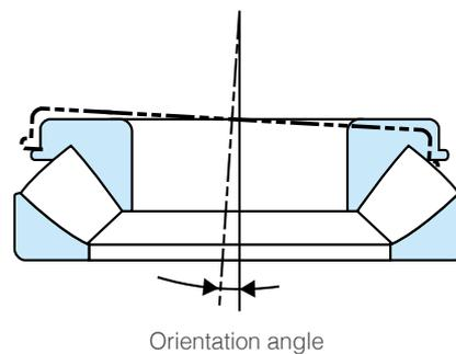
**Lubrication:** thrust spherical roller bearings are usually heavily loaded and must be lubricated with oil. Due to the internal construction of these bearings, grease lubrication is only possible at low speeds and with limited loads.
