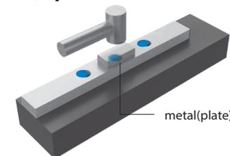
Continue pounding the cap until the cap is on the same plane with the top surface of rail.
