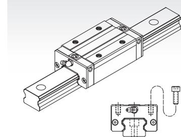
All dimensions are same as SME-SA except the mounting hole dimensions of carriage are different and the height is lower, which do not change the basic loading rating.
