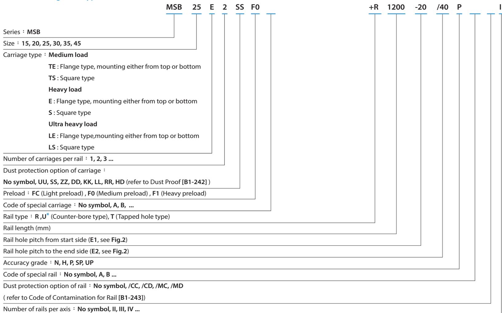
**Note\*** : U type rail is only applicable for MSB15 with M4 mounting hole.
