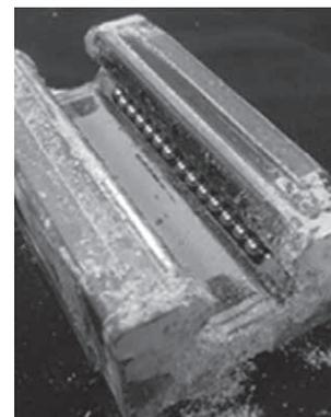
After running 150 KM in a wood flour test environment, the carriage is still moving smoothly and the steel balls are also glossy. The end seal and inner seal protect against wood flour from entering the carriage. Overall running smoothness is not effected.
