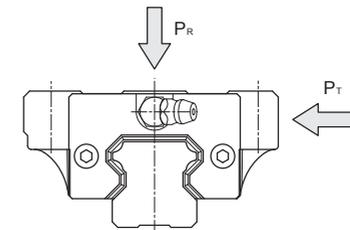
For the case of mono rail, the moment effect should be considered. The equation is:
