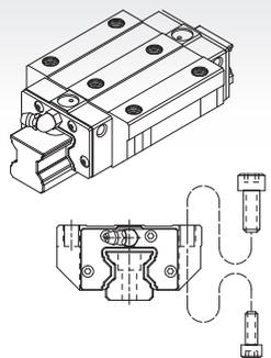
This type offers the installation either from top or bottom side of carriage.
