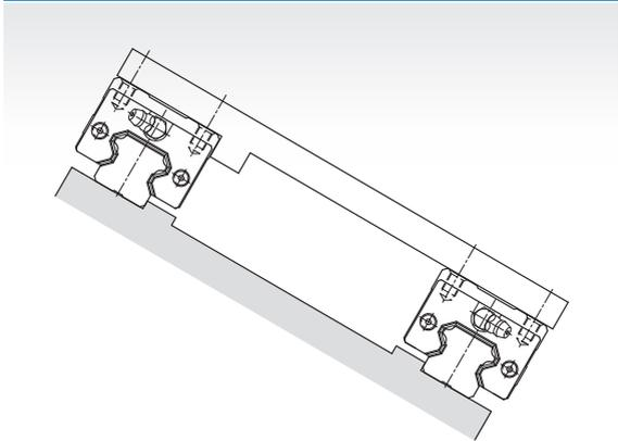
**Fixing Methods of Linear Guideway**
