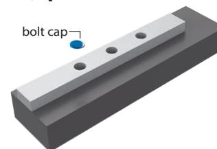
Put the cap into the bolt hole of rail.
