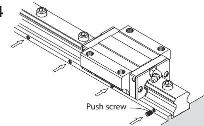
Tighten the push screw in sequence to ensure the rail close matching the reference side of bed.
