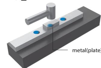
Put the plate on the cap, then pound it into the bolt of rail with rubber hammer vertically.
