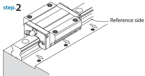
Gently place the linear guideway on the bed, and pushing it against the reference side of bed.
