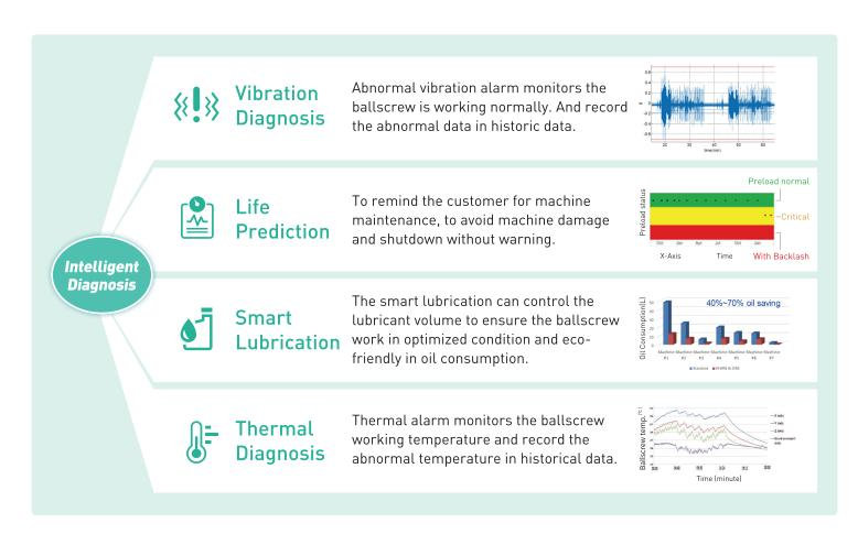
i4.0BS® transmits signals via sensors and PLC I/O to the edge computing module for calculation and analysis. Then the results are shown on display devices through Ethernet network to achieve remote monitoring.
