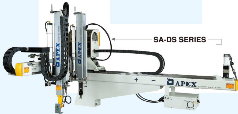
Cable guide protection on all electrical wires and air hoses.
