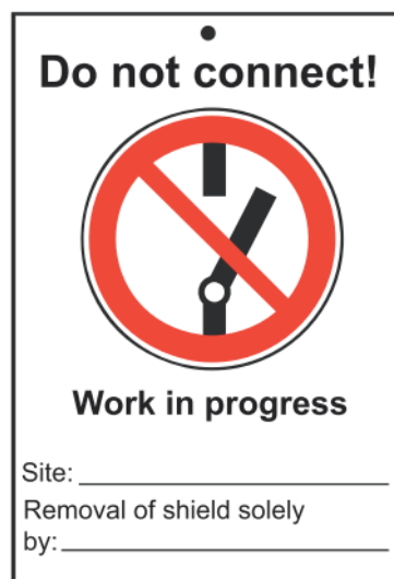
Fig. 7.2 Example of a warning sign
