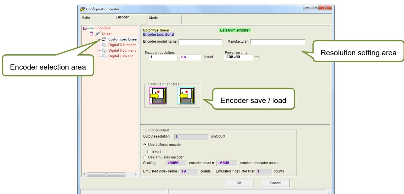
Figure 5.2.2.2.1 Encoder configuration page for customized encoder
