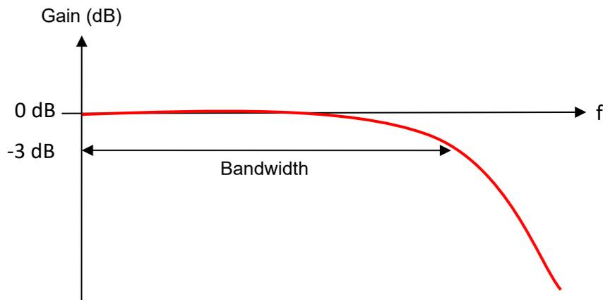
Figure 3.6.2.2 Bandwidth of Bode plot
