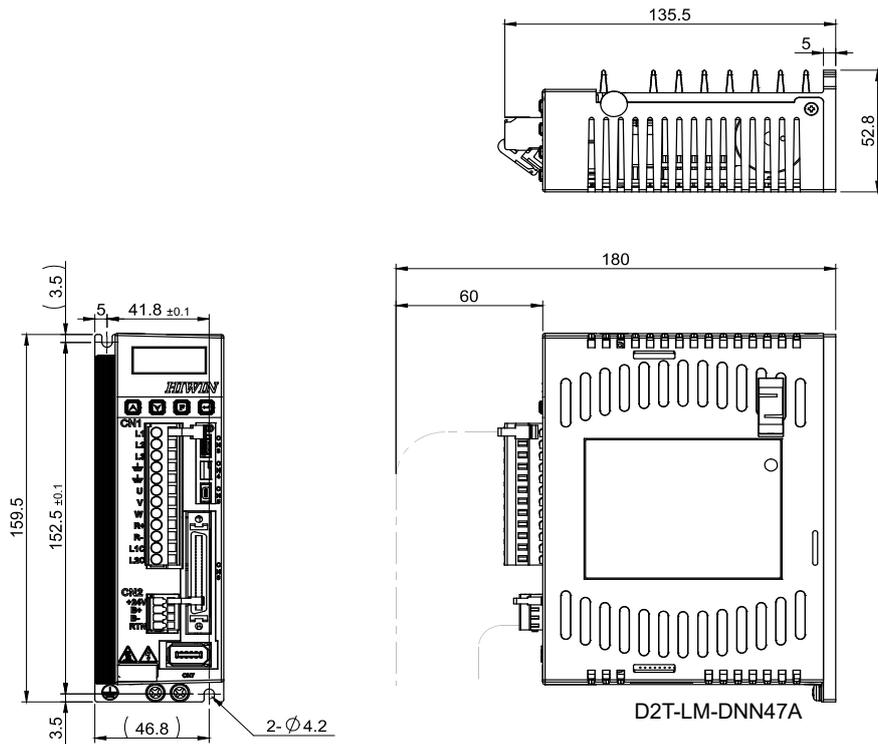
Figure 2.3.1 Dimensions of D2T-LM Frame B (Standard)
