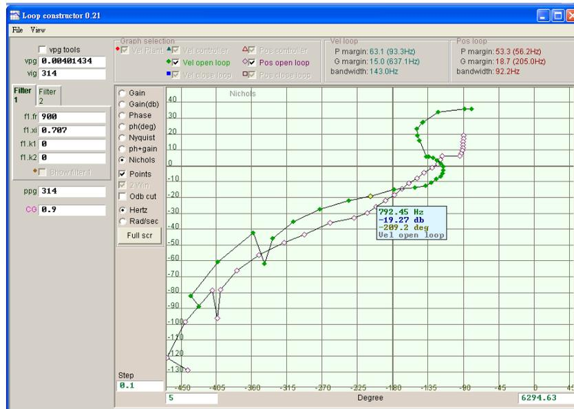
Figure 6.7.2.4.1 Nichols plots of Vel open loop and Pos open loop
