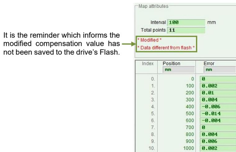
Figure 6.9.1.2 Parameter setting of error map
