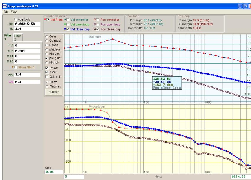
Figure 6.7.2.3.1 Bode plots of Vel close loop and Pos close loop
