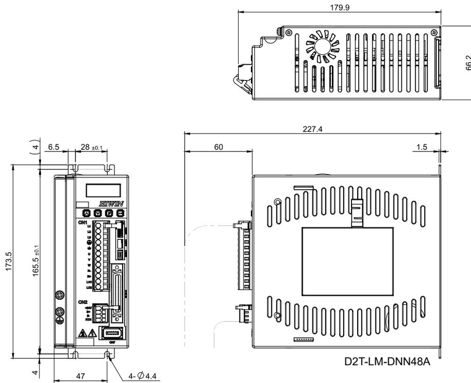
Figure 2.3.2 Dimensions of D2T-LM Frame C (Standard)
