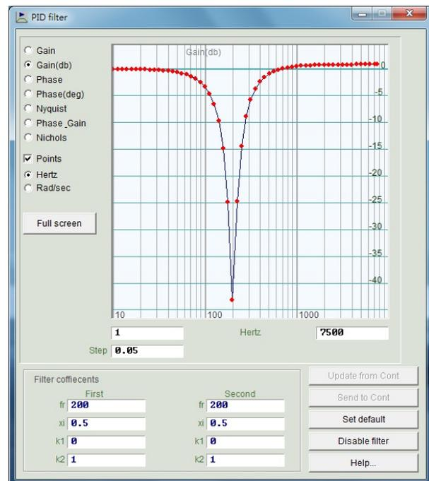
Figure 6.6.1.3 Notch filter
