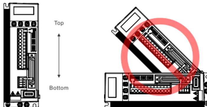
Figure 2.4.1 Correct and incorrect mounting directions
