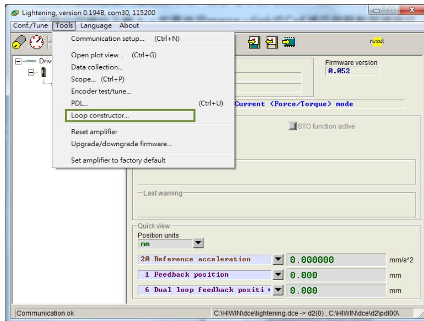
Figure 6.7.1 Open “Loop constructor” from “Tools”
