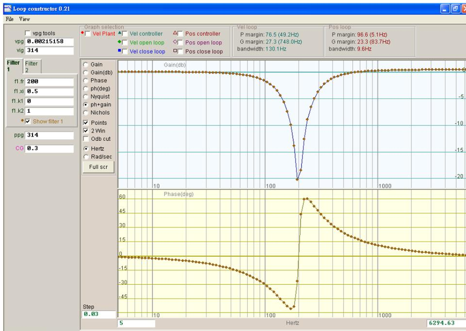
Figure 6.7.3.2.1 Notch filter
