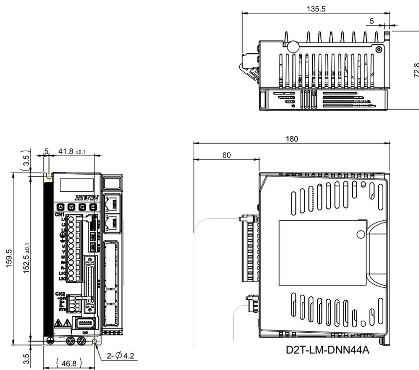
Figure 2.3.3 Dimensions of D2T-LM Frame B (Fieldbus)
