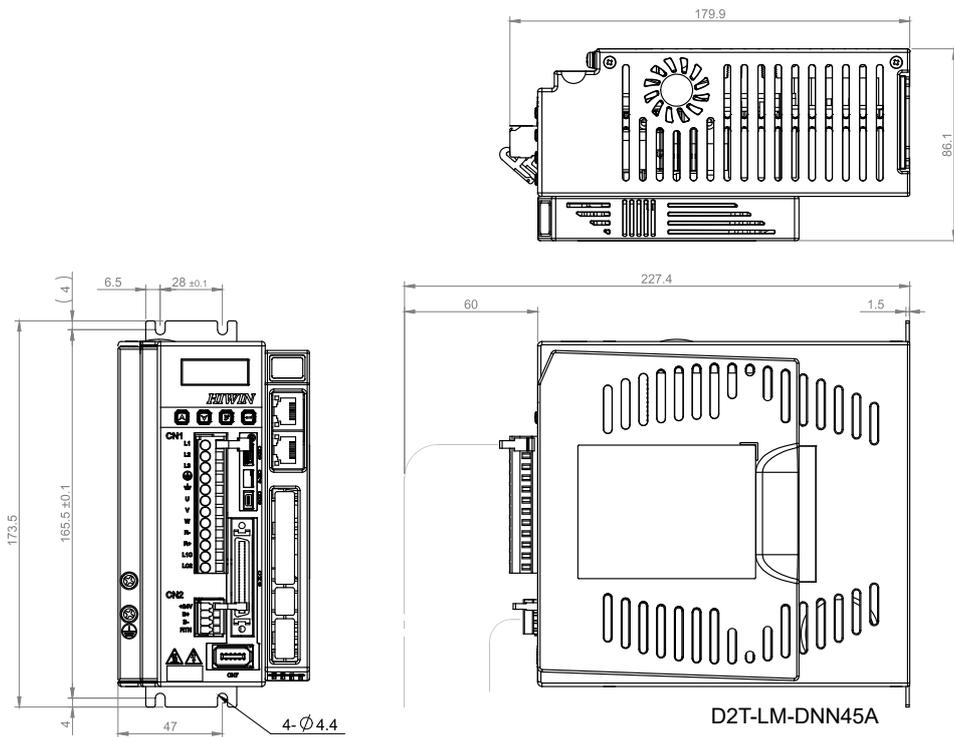
Figure 2.3.4 Dimensions of D2T-LM Frame C (Fieldbus)
