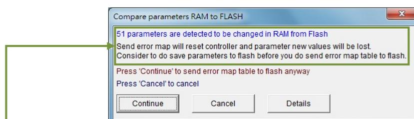
Current parameters except error map parameters are different from those in the drive's Flash. If users click the “Continue” button to save error map parameters to Flash, servo parameters will be lost due to the forced “Reset” action of the drive.
