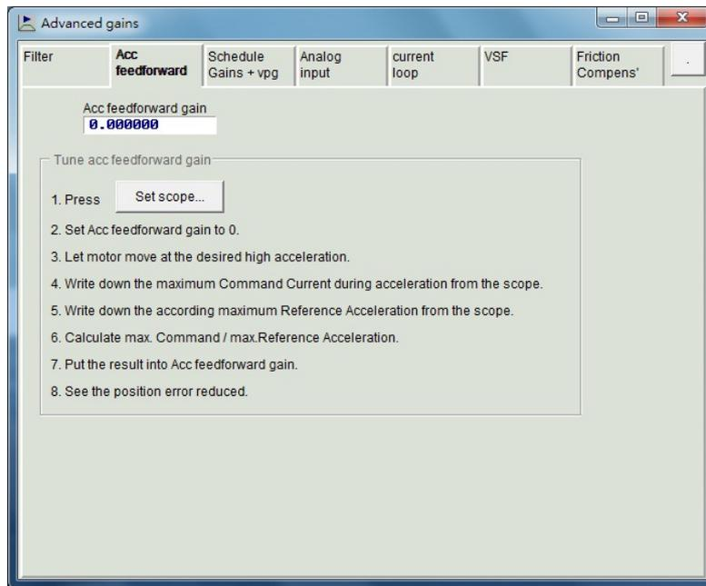
Figure 6.6.2.1 Acceleration feedforward
