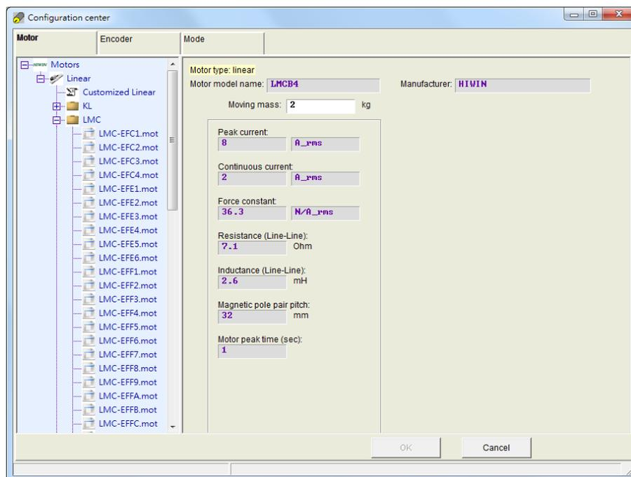
Figure 5.2.1.1 Motor configuration page for Lightening 0.194B or above
