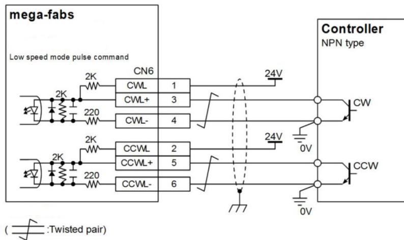
Figure 4.6.1.6.2 Wiring example for converting single-ended negative logic to positive logic CW/CCW signal
