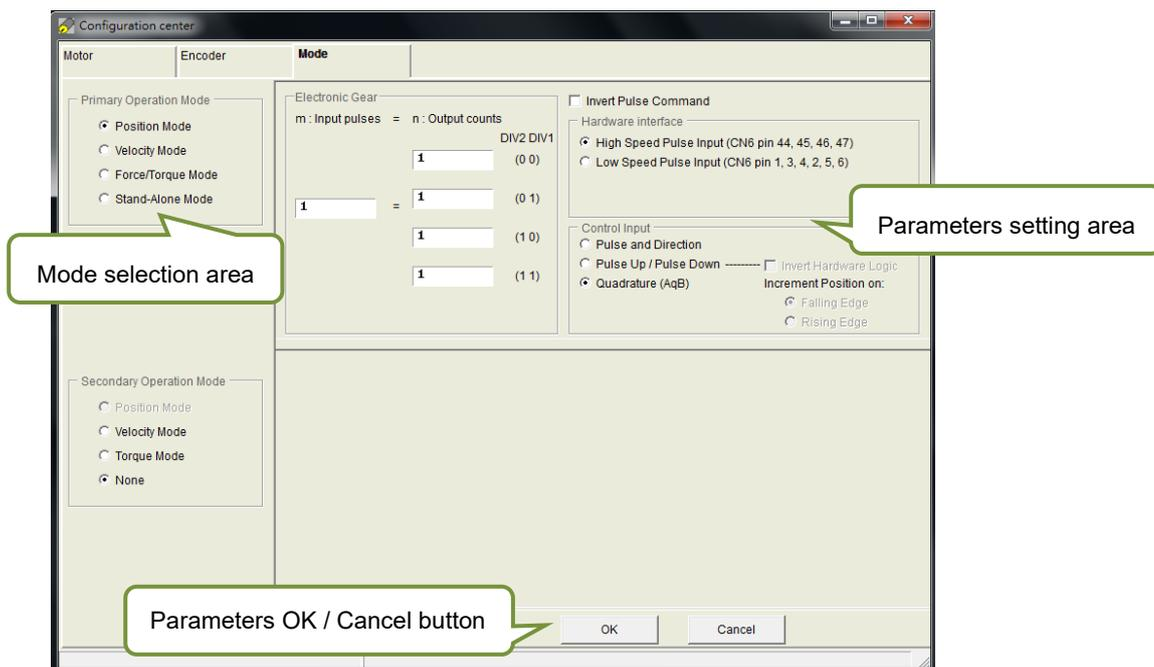
Figure 5.2.3.1 Operation mode configuration page
