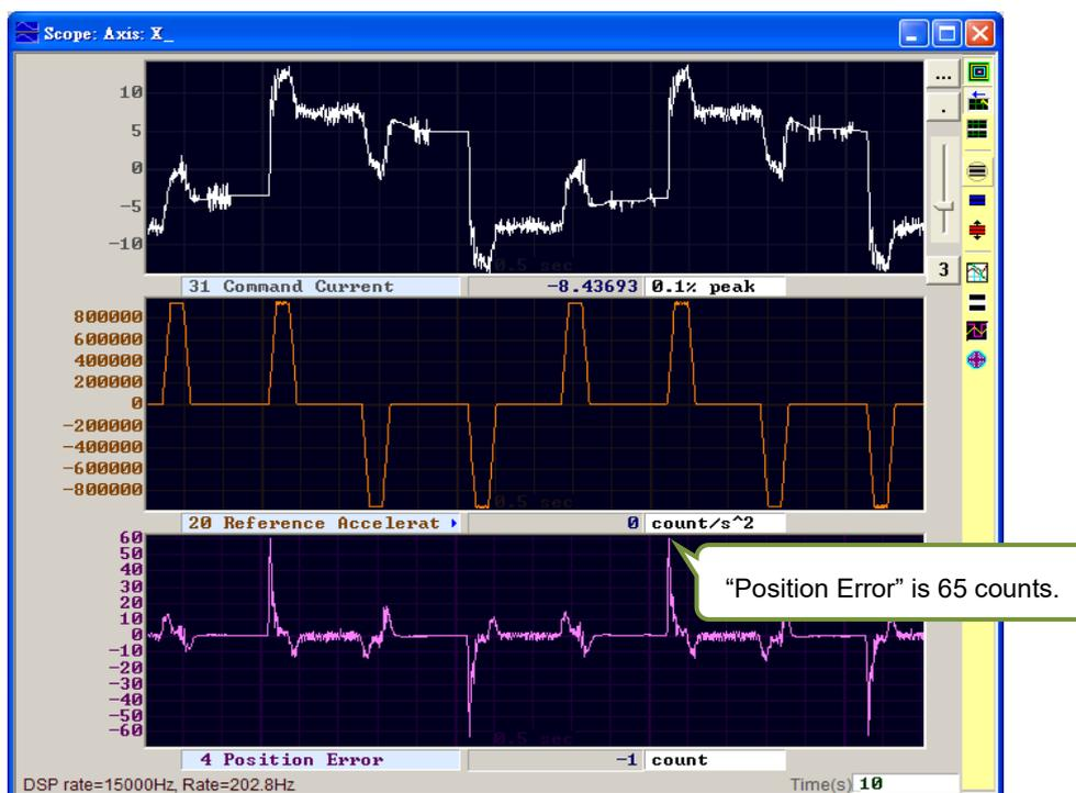
Figure 6.6.2.4 Result of adding acceleration feedforward
