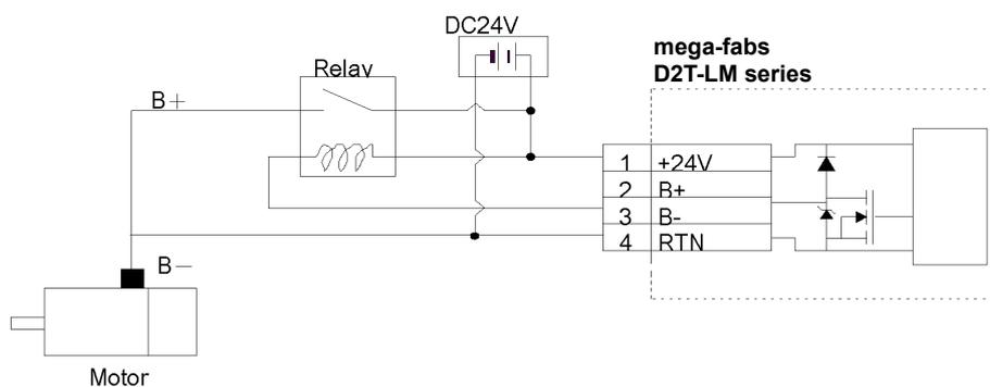
Figure 4.1.3.2 CN2 brake wiring (with a relay)
