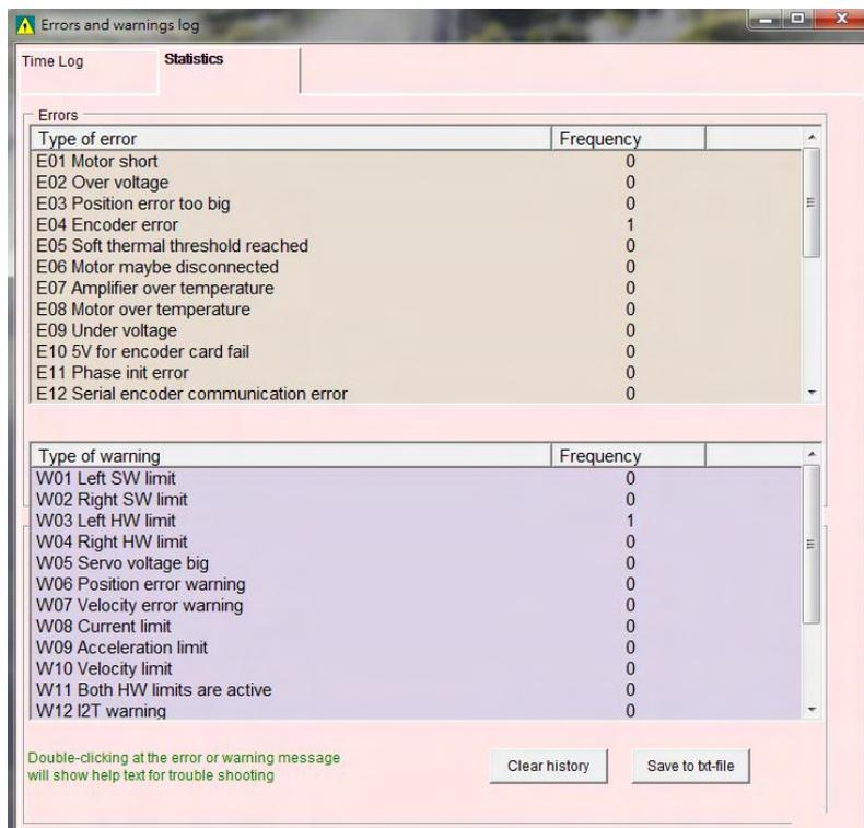
Figure 9.2.2.3 Statistics in “Errors and warnings log”
