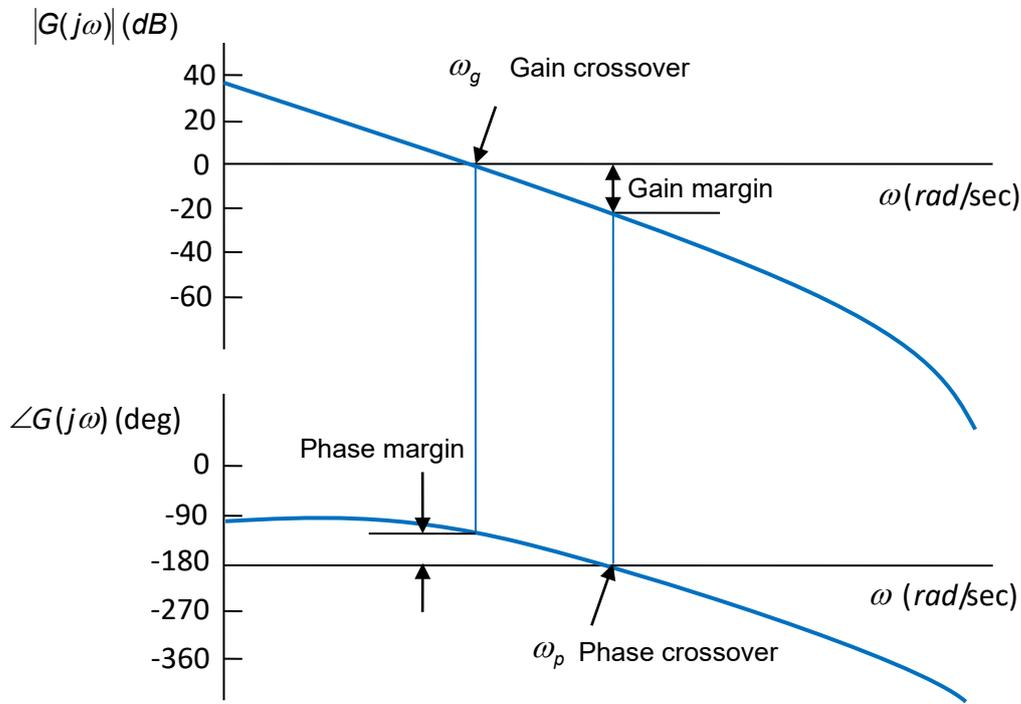
Figure 3.6.2.1 Gain margin and phase margin of Bode plot
