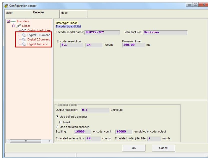
Figure 5.2.2.1.1 Encoder configuration page for standard encoder
