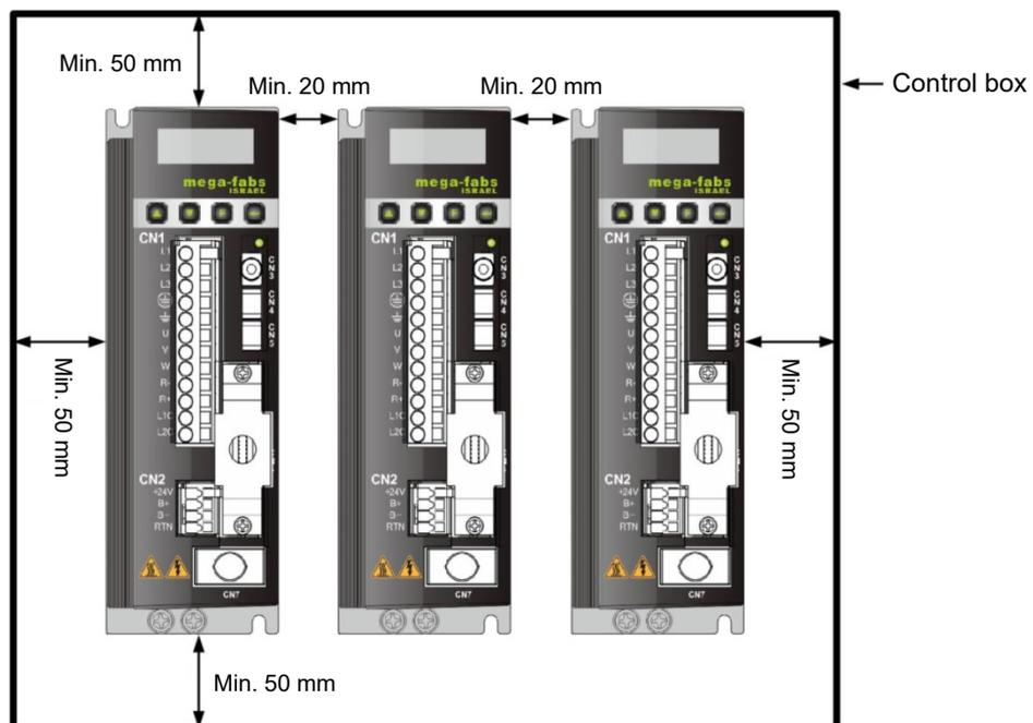
Figure 2.4.2 Installing multiple servo drives
