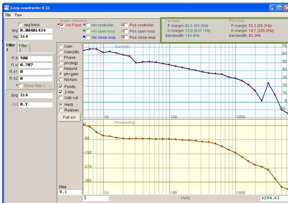
Figure 6.7.5.1 Loop constructor – P margin and G margin
