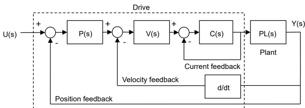
Figure 6.7.2.1.1 Control architecture of the drive
