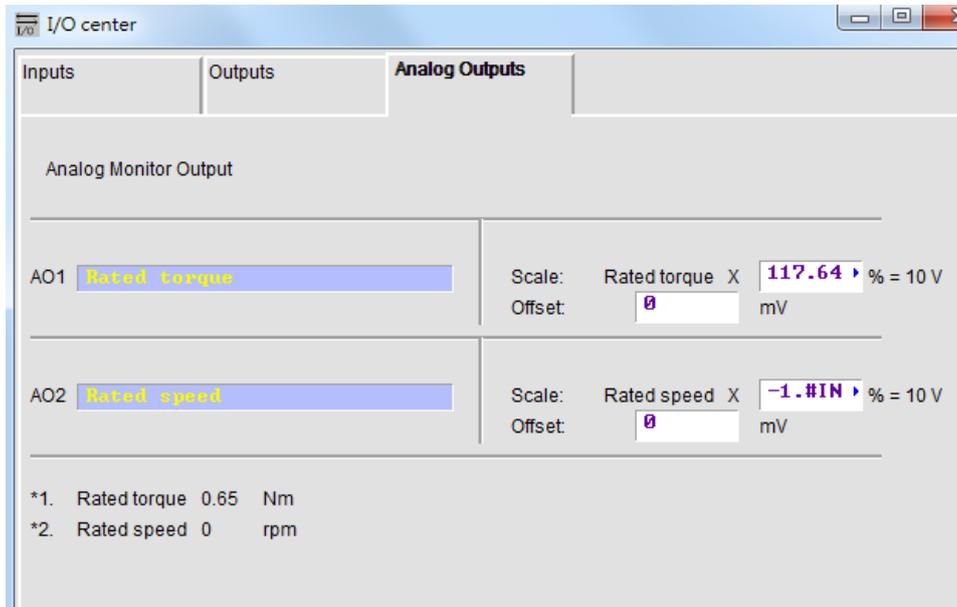
Figure 5.4.3.1 Analog output configuration page
