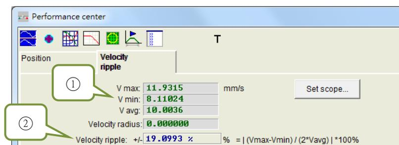
Figure 6.2.2 Performance center – "Velocity Ripple" tab
