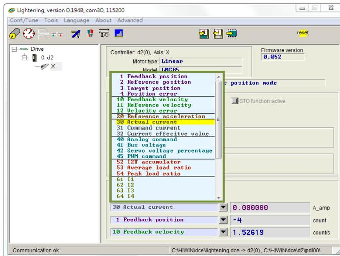
Figure 6.1.2.1 Physical quantity menu in “Quick view”
