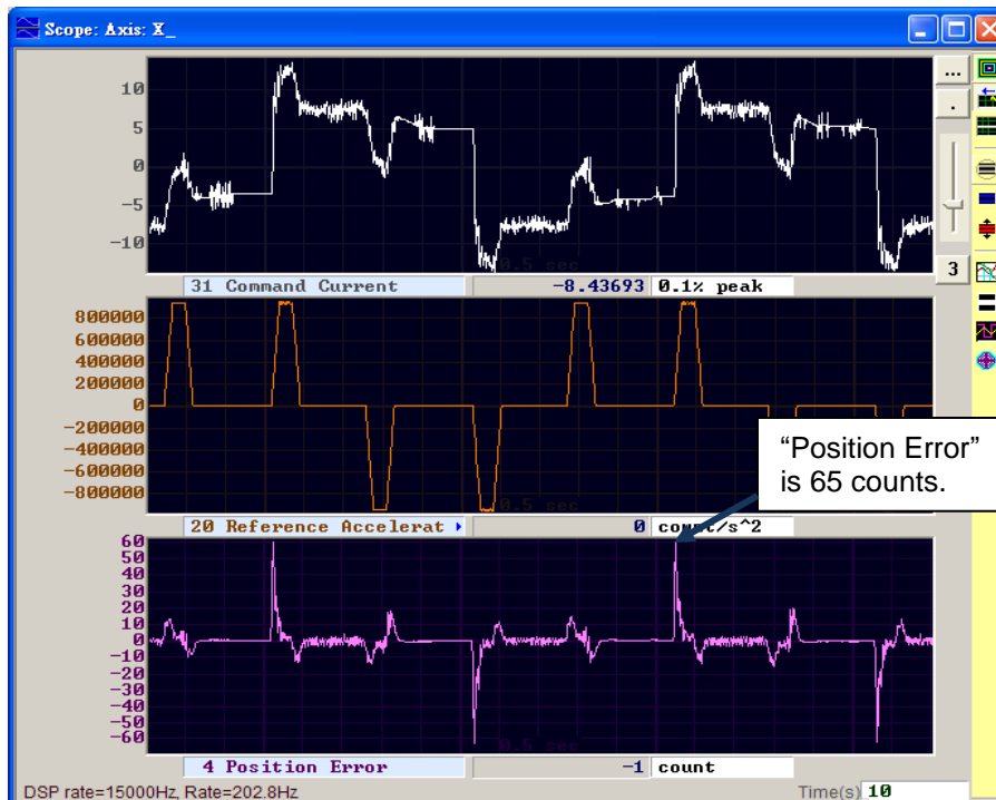
Figure6.6.2.4 Result of adding acceleration feed-forward
