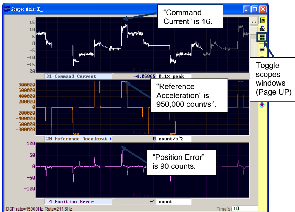
Figure6.6.2.2Trajectory result of motor movement
